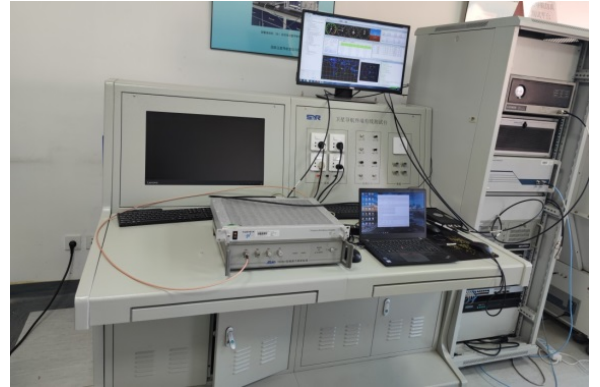
Fig.6. GNSS receiver absolute calibration
